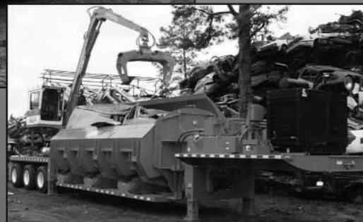
The 580 CL is truly the heavy weight in portable Balers and Loggers. This fully automatic, one man machine can produce over 200 tons per day. The new 19' 3" L box design enables you to load and unload loose sheet metal and car bodies with ease. The portable 580 Car Logger weighs in at 92,000 pounds, and produces a load every 30 minutes.
