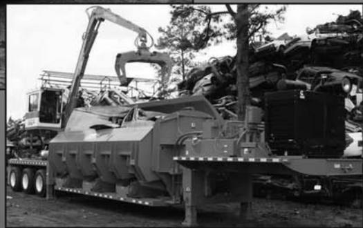
The 580 CL is truly the heavy weight in portable Balers and Loggers. This fully automatic, one man machine can produce over 200 tons per day. The new 19' 3" L box design enables you to load and unload loose sheet metal and car bodies with ease. The portable 580 Car Logger weighs in at 92,000 pounds, and produces a load every 30 minutes.
