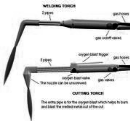
The top torch is a welding torch and the bottom is a cutting torch
