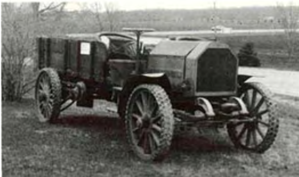
This 1910 Avery truck is all original. This combination truck-tractor had a pulley on front of engine to run belt for a threshing machine. Built mostly for agricultural use.
